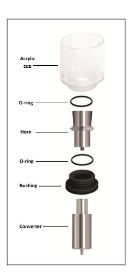
Though it is unlikey, the cup horn and converter connection can loosen over time.
