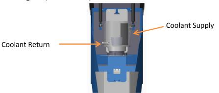
Cold water (Supply) enters from the Chiller to the top right side of the cup. Water exits (Returns) from the lower left side back to the Chiller.
