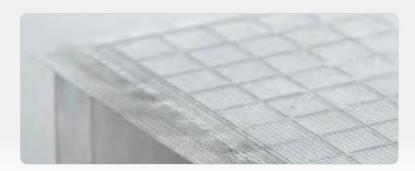
This adhesive seal is perforated with micropores so that it is permeable to gases but provides a barrier to bacteria and other solid contaminants. The gas permeable seal is a convenient option for covering cell cultures and can be pierced or peeled without any remaining sticky residue.
