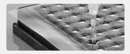
This strong adhesive seal was developed to facilitate easy sample removal with a manual or automated system. The seal is a transparent polyester film with a strong adhesive layer. 96 adhesive free windows have been cross-cut. This enables access to the sample wells with a tip or probe with minimal pressure.
