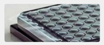
This is a strong adhesive seal that has 96 or 384 adhesive free windows. These windows allow air and CO<sup>2</sup> exchange, but prevent moisture evaporation from the sample.
