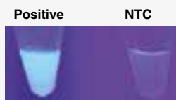
Visualization using a fluorescent intercalating dye (e.g., ethidium bromide, SYBR® green or calcein/HNBlue)
