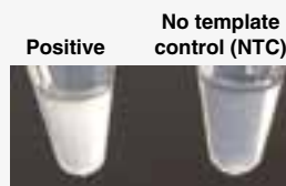
LAMP product is visible by eye due to the precipitation of magnesium pyrophosphate
