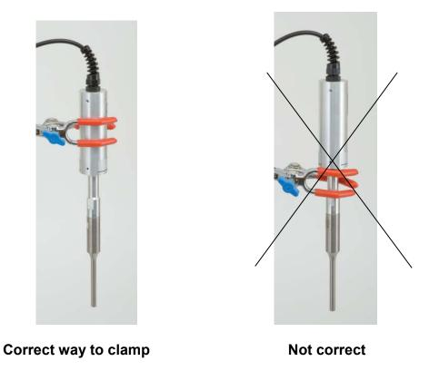
Note: Using a Qsonica sound enclosure or stand will ensure a proper fit.
