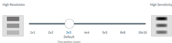
**Fig 11.** The CCD detector of ImageQuant 800 imager allows for on-chip binning. Default settings (5×5 for upper and 3×3 for lower tray position in chemiluminescence mode) can easily be changed using the slider. Low binning levels improve the resolution and high binning leads to shorter exposure times.
