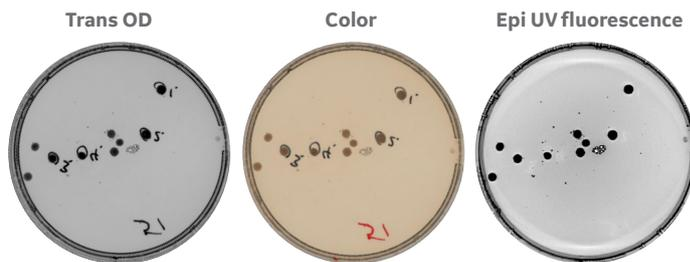
**Fig 18.** Different imaging modes are available for imaging of colonies on petri dishes. Optical density measurements (left) provide a direct measurement of the OD of each colony. It is also possible to get color images (middle) and do epi-fluorescence imaging. For example, UV-imaging (right) was done to capture the auto-fluorescence of the cells. With the NP lens accessory, chemiluminescence imaging is also possible using an ImageQuant 800 imager.
