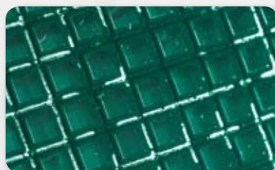
Figure 3: Competitor's plate showing areas with no adhesive
