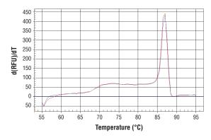
PCR product melting curves were obtained for real-time PCR reactions performed using SimpleChIP® Human tRNA-Leu Anti-Codon (TAG) Primers. Data is shown for both duplicate PCR reactions using 20 ng of total DNA. The melt curve consists of 80 melt cycles, starting at 55°C with increments of 0.5°C per cycle. Each peak is formed from the degradation of a single PCR product.
