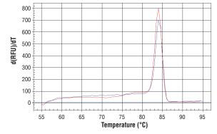
PCR product melting curves were obtained for real-time PCR reactions performed using SimpleChIP® Human Axin2 Intron 1 Primers. Data is shown for both duplicate PCR reactions using 20 ng of total DNA. The melt curve consists of 80 melt cycles, starting at 55°C with increments of 0.5°C per cycle. Each peak is formed from the degradation of a single PCR product.
