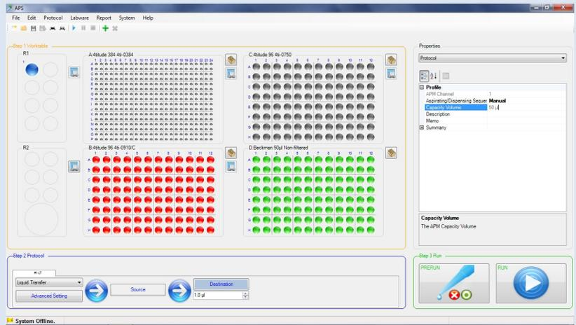
**Figure 3: Automate loading 384 DNA samples from 4 x 96-well PCR plates to 384-well PCR plates with the 4LAB™**
